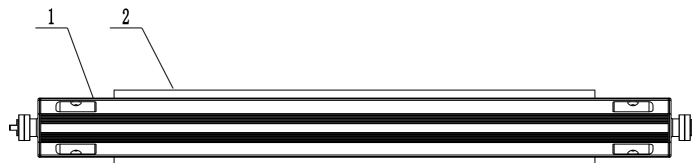
1. Rewind shaft 2. Cardboard rewind
