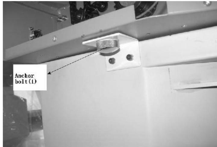
2. Insert four (4) anchor bolts through the stand into the bottom of machine
